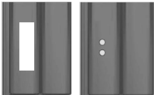
sleuf/gaten in dakpan ca 75 x 175mm
